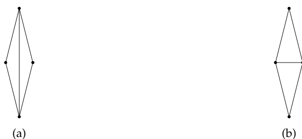
Figure 2.10: A quadrilateral is triangulated in two different ways. (a) A quadrilateral is triangulated into two skinny triangles. (b) A quadrilateral is triangulated into two better-shaped triangles comparing to (a).
