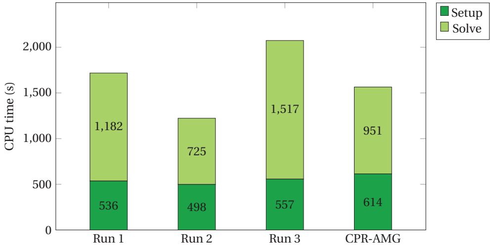
Figure 3.6: SPE9 without capillary pressure: LS CPU time (s) breakdown.
