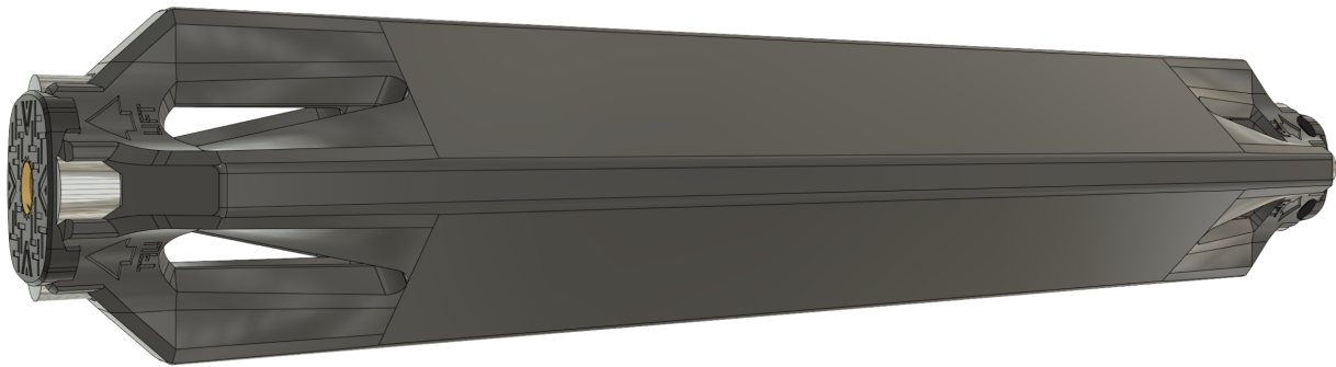
Figure 4.6: Design of a slender truss building block.
