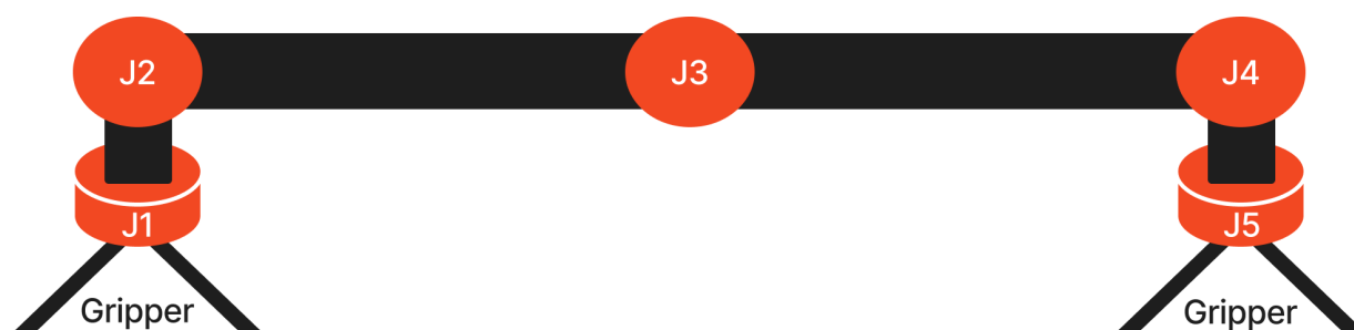
Figure 5.1: Joint configuration of an inchworm locomotion lattice assembler.
