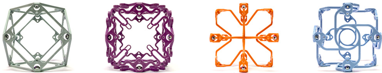
Figure 2.10: Metamaterial unit cells. From left to right; Stiff, compliant, auxetic and chiral. Figures courtesy of [25].
