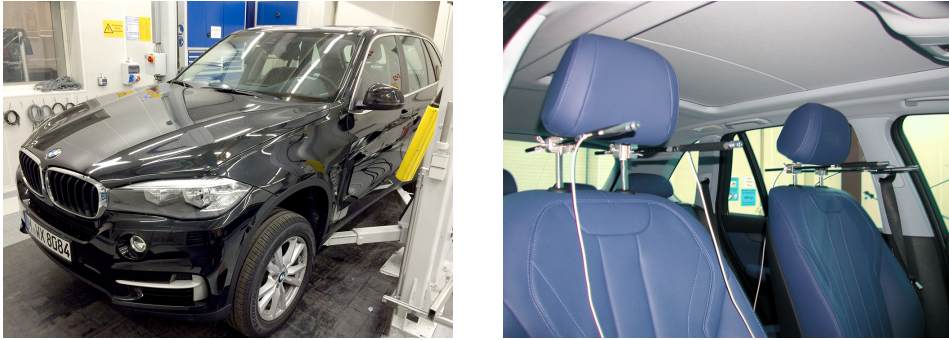
Figure 9.8: Impression of the vehicle that was used for FRF and operational measurements. The photo on the right shows the four microphone positions in the interior.
