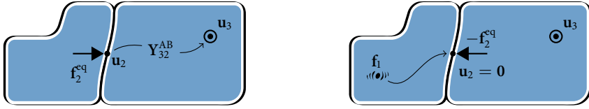
(a) Application of equivalent forces to the passive system AB, representing the operational excitation.
