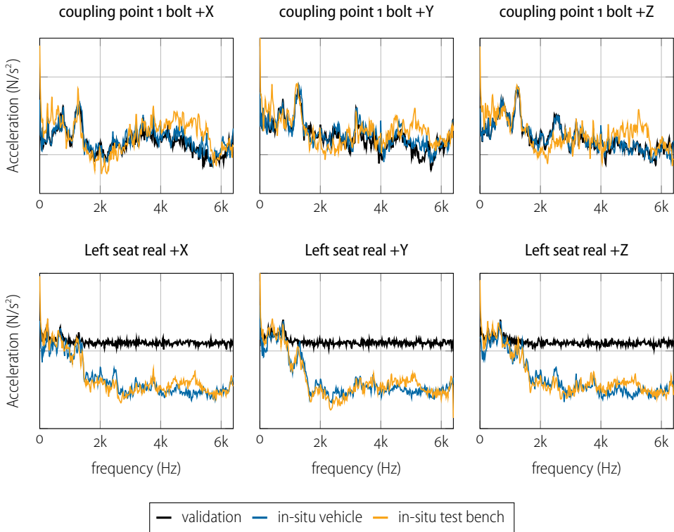
Figure 9.14: TPA prediction of structure-borne responses at a sensor underneath coupling point 1 (top) and at the left seat rail inside the vehicle (bottom).
