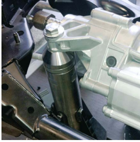
(a) Stiff test bench support with 3D force sensor clamped in near the interface.
