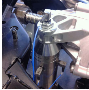
(b) Stiff test bench support with four additional tri-axial accelerometers.
