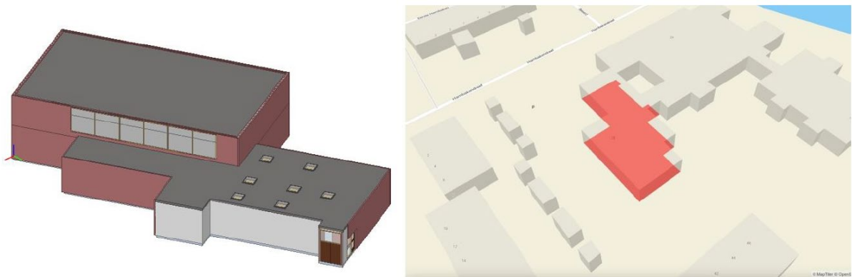
Figure 3. 3D view of a georeferenced BIM model (left) and its visualisation on the map (right).
