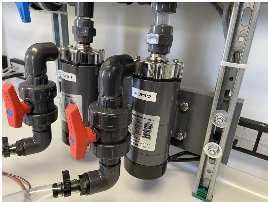
Figure 4.2: Magnetic impeller drive pump. Each pump is 25 W, has a maximum flow rate of 19 L/min, and circulates the anolyte/catholyte from the gas tank to the stack. The pump has a 6.5 cm diameter and 16.5 cm length.
