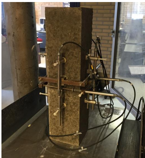
Figure 6.1 Testing set-up for elastic modulus measurement on AAS and AASF concrete.
