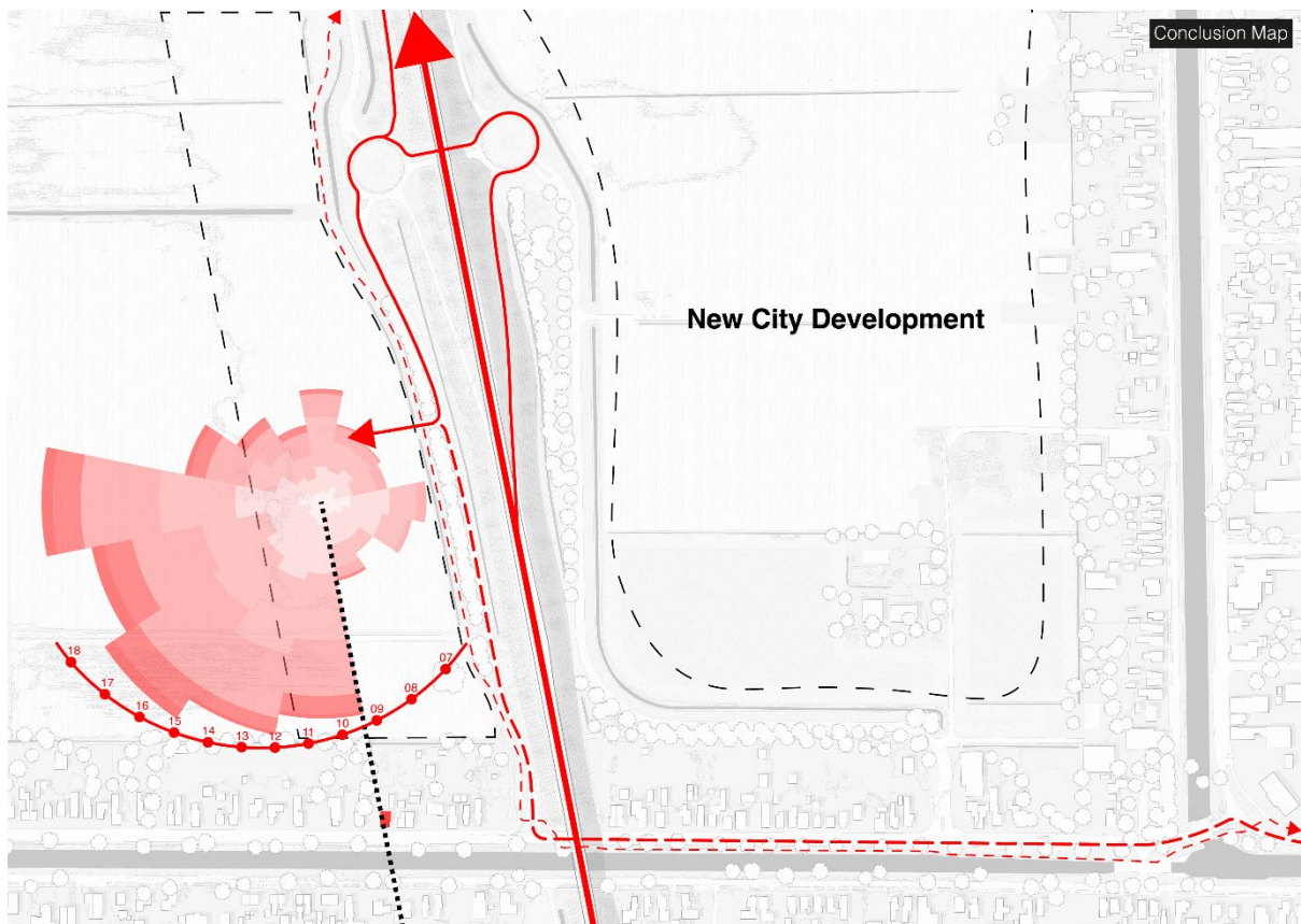
Figure 4. Site analysis diagram: N366 talud, COA pedestrian route, railway alignment, wind direction, and site ground level relative to the N366.
