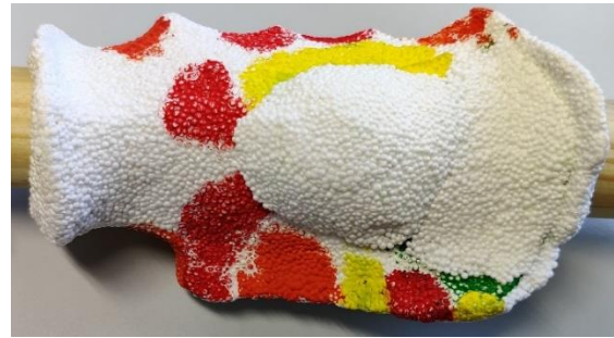
Image 36: Foam clay prototype with a print of the PDT map and added material on the high PDT regions.
