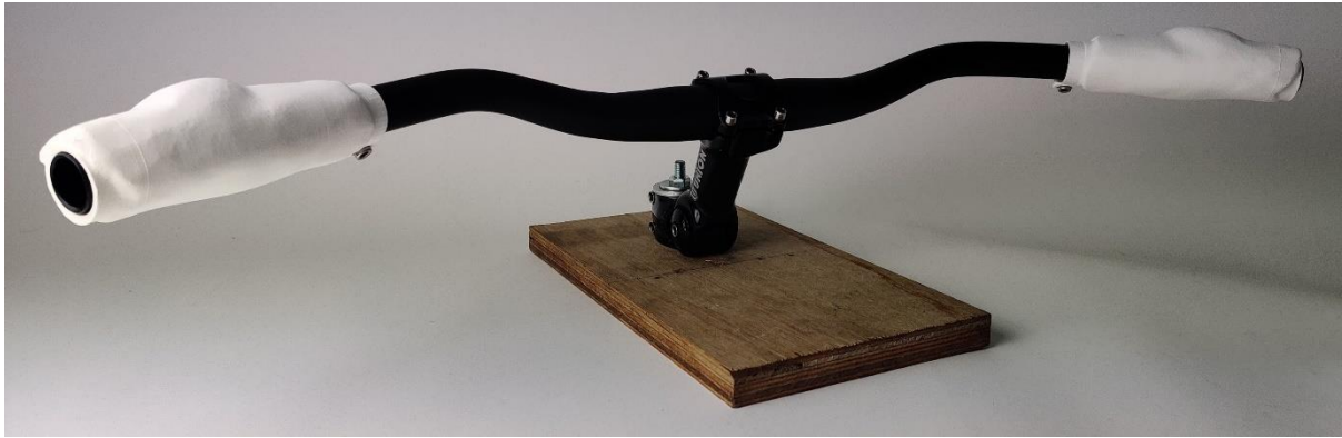
Image 47: Handlebar standard made for physical assessment.
