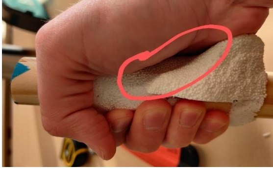
Image 45: The resulting gap when testing a concept based on a 45° handlebar at 30°.
