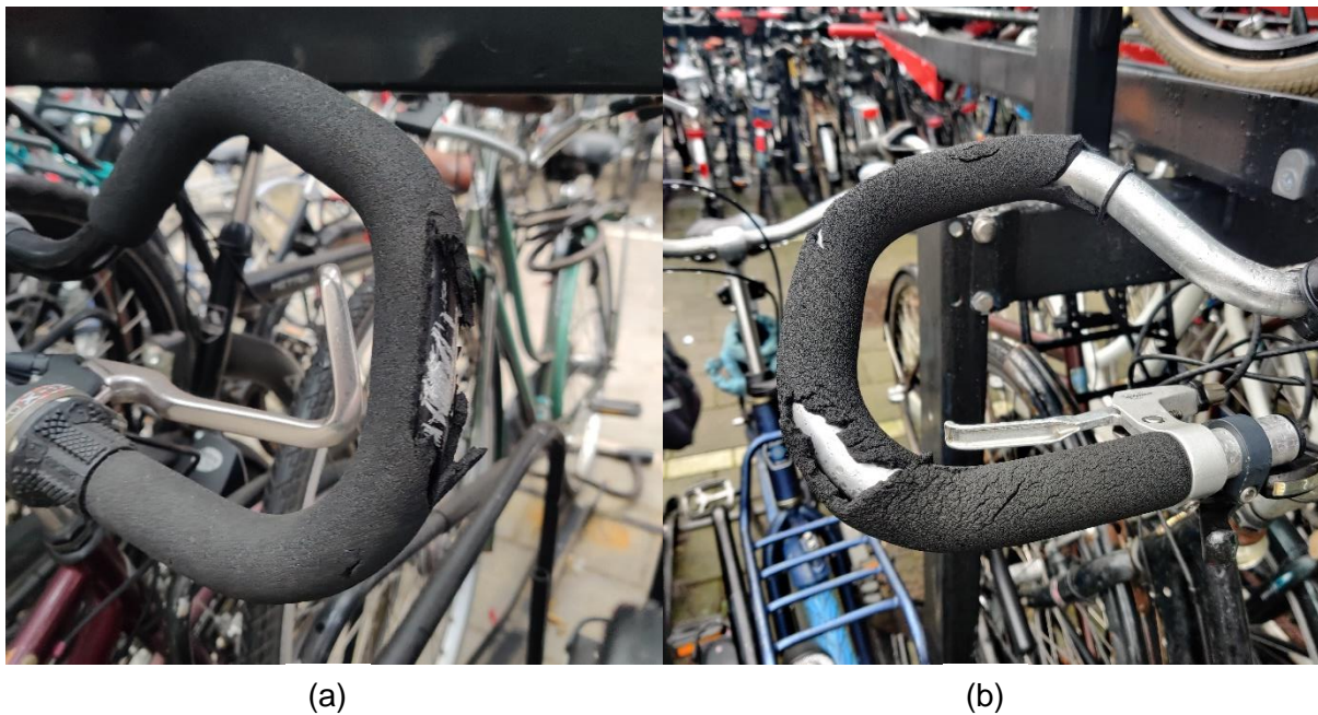
Image 23: photographs showing alternatively shaped handlebars damaged by impact (a) and wear (b).
