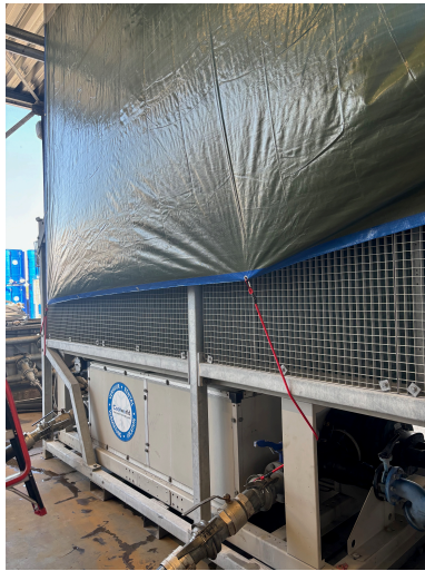
(a) Bulging with one side of the sail closed the elastic attachment was not solid enough.
