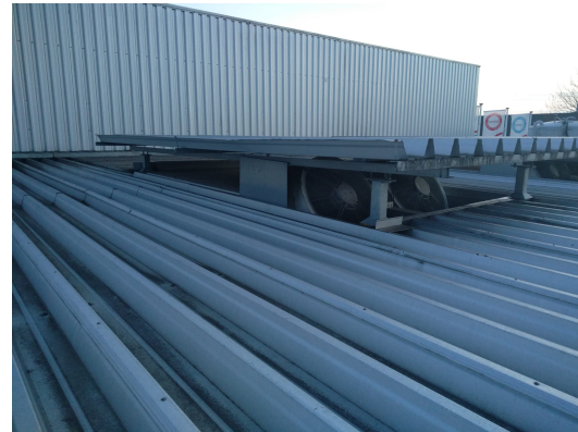
(b) The positioning of the fans in the roof section of the testing facility.
