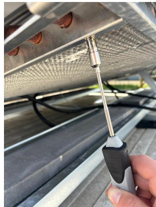
(b) Testo 922 temperature probe for temperature
