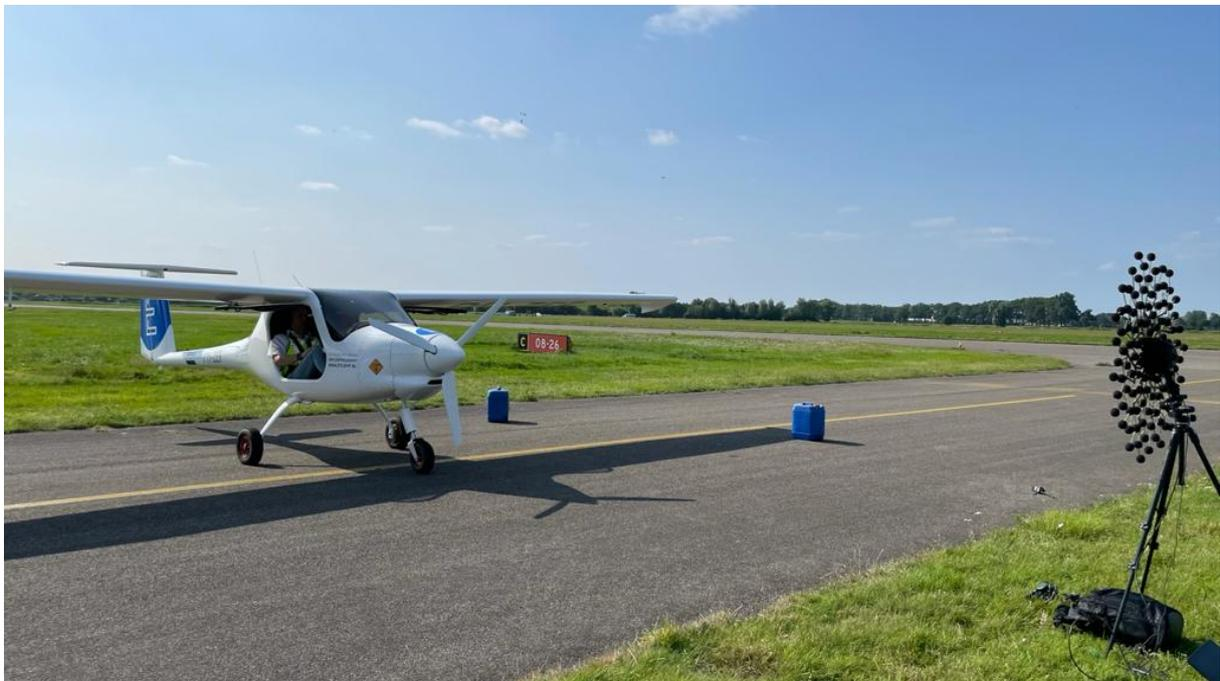
*Figure 3: Setup engine run-up with the microphone array aligned with the propeller rotation centre.*
