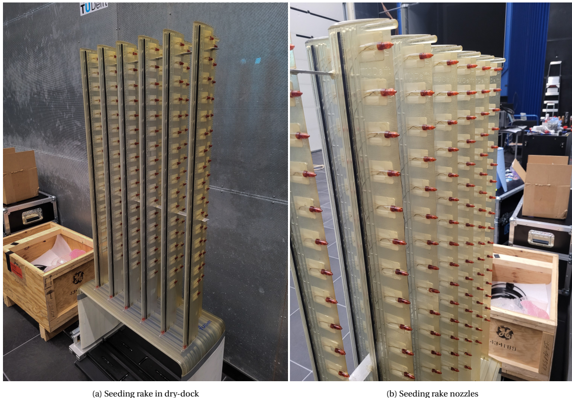
Figure 3.6: The seeding rake used to produce the bubble stream in dry dock
