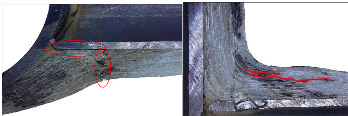
Fig. 23. Cut-through 90° small-scale wrapped composite joint specimens loaded in bending.
