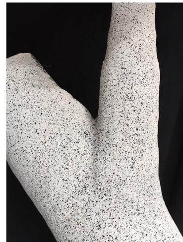
Fig. 6. The 3D DIC system with live measurement of displacements and strains on the surface of specimen at two scales.
