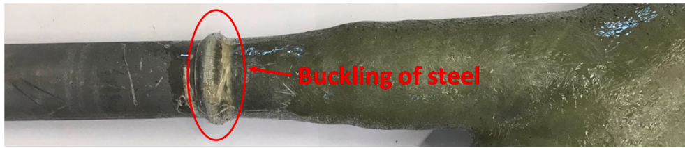
Fig. 15. Buckling of brace outside the composite wrap in compression test.
