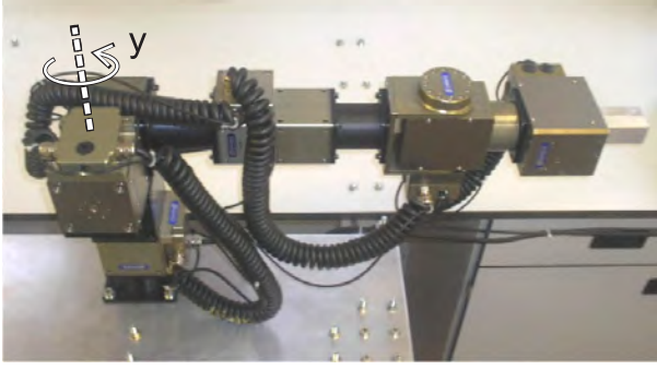
Fig. 4. Robotic manipulator system showing actuated output, y .
