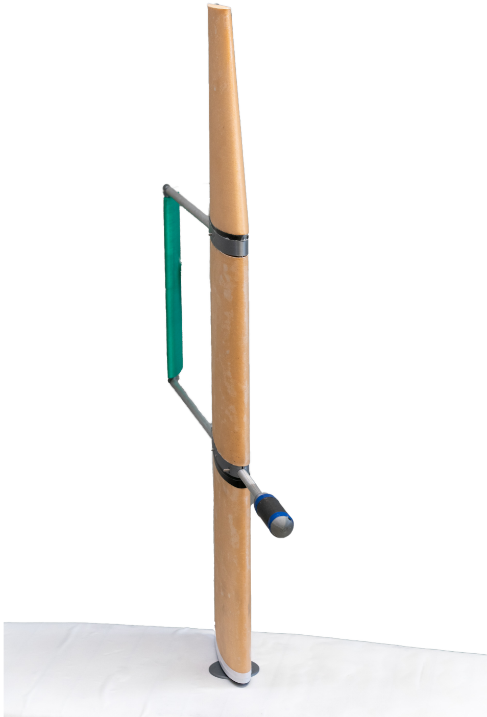
Figure 6.25: A close-up of the prototype sail from the direction of the incoming airflow shows that the main wing is pitched slightly to generate lift to the right. This orientation is controlled by the tailwing, which is angled oppositely to the flow and sets the main wing's angle of attack.
