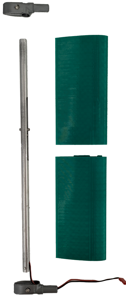
(a) An overview of the parts that make up the tailwing. The linear actuator (visible in Figure 6.13) is housed in the tube. It moves a pin up and down a milled slot. This pin interfaces with an elongated helical cutout inside the green wing, which rotates by 60^\circ over a length of 40mm.
