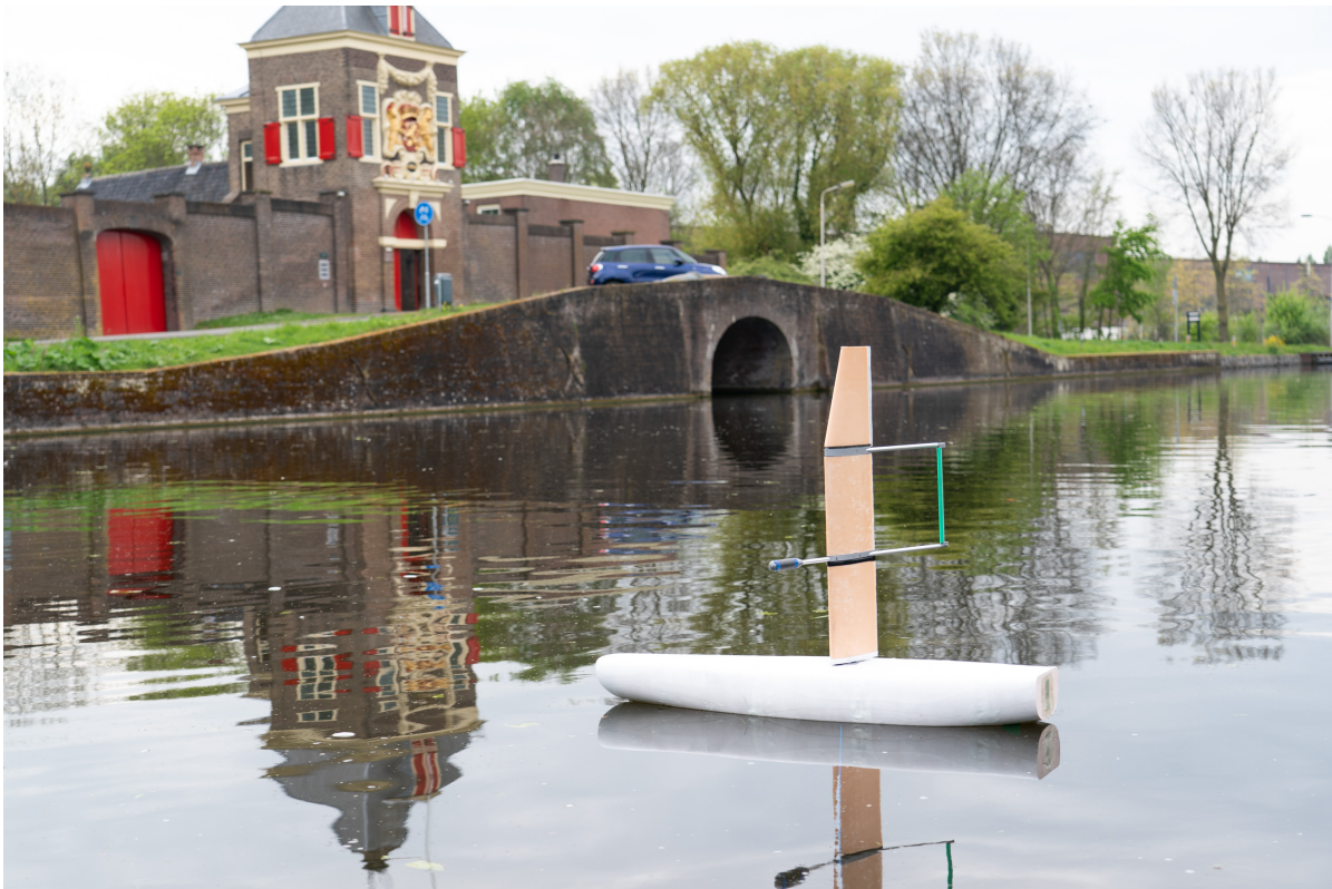
Figure 6.27: The trim (longitudinal placement in water) of the SDC25 appears perfect by eye, but is off by 6mm after evaluation.
