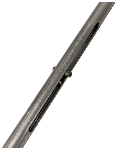
(b) A close look at the pin and slot. The linear actuator moves the pin up or down.
