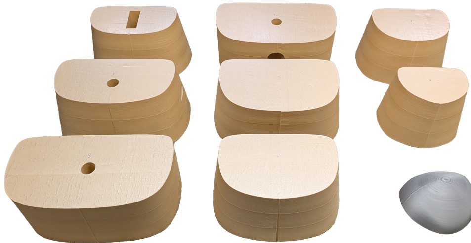
Figure 6.20: All 8 hull sections and bow, aligned from stern to bow, from top to bottom, and left to right. Holes have for the mast/keel, the electronics compartment, and cable routing have also been cut.
