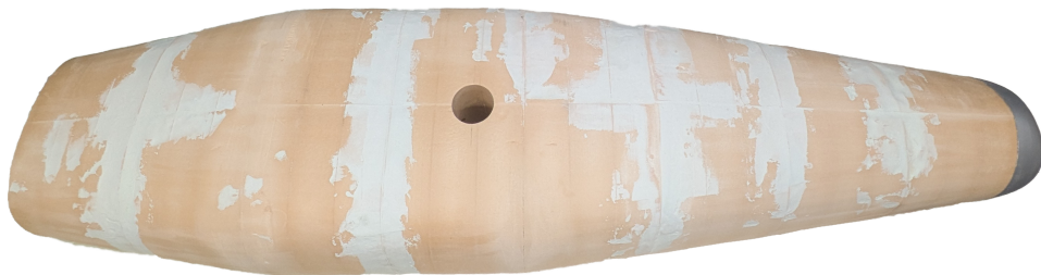
Figure 6.22: The hull after gluing, filling, and sanding. In hindsight, using a two-component epoxy filler to close small gaps was a mistake. The heat generated during curing caused dents in the foam wherever excess filler was applied, leaving the surface in a worse condition than before. Simply sanding would have yielded a better result. The gaps themselves were due to about half of the sections being cut using an earlier version of the toolpath code which had mismatched point pairs, though these sections were still deemed usable.
