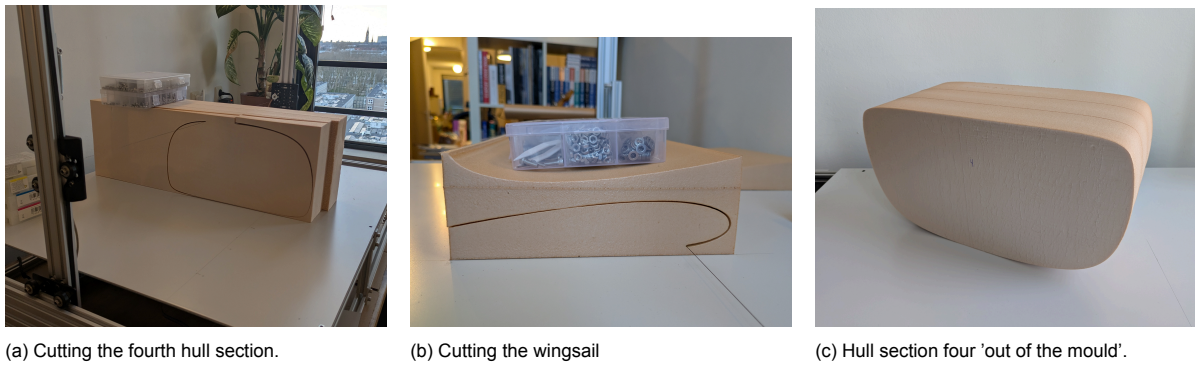
Figure 6.19: Examples of cutting parts of the hull and sails with the hot wire CNC foam cutter.
