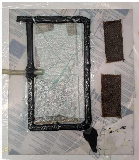
Figure 5.12: Manufacturing of the four sample pieces. Two are cured under vacuum, two under normal atmospheric conditions with periodic heating with a heat gun.
