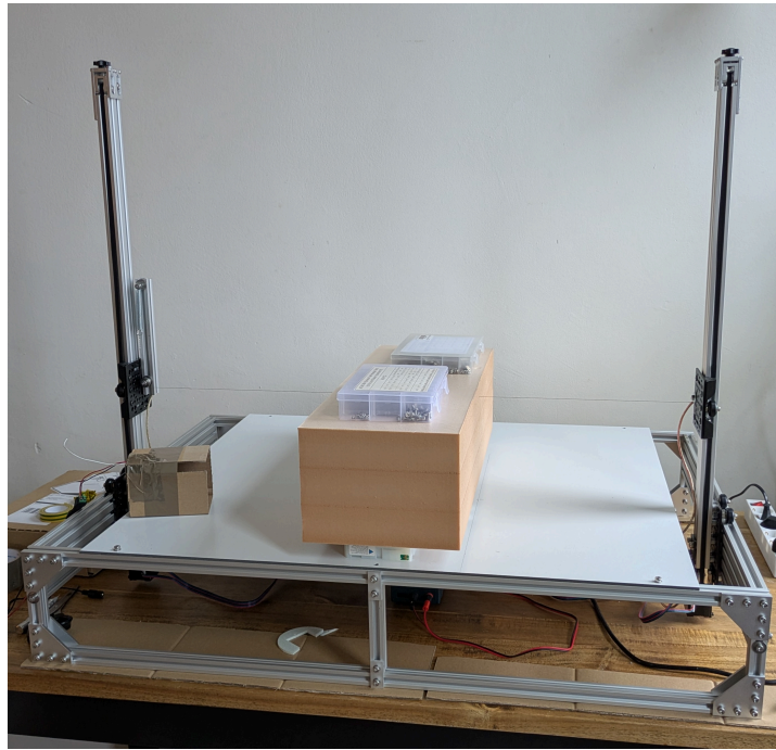
Figure 6.17: The hot wire CNC in use, squaring up a foam blank. Small weights are placed on top of the foam to keep it in position in case the wire exerts a slight pull on it.
