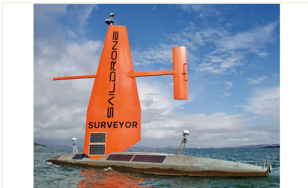
image / figure 2 An uncrewed sailing vehicle developed by Saildrone for the open oceans, length = 22m. (Saildrone, 2015)
