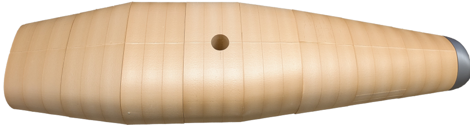
Figure 6.21: All hull sections placed in order, before glueing.
