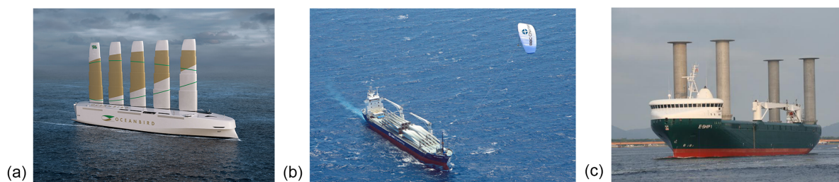
Figure 2.6: Sail assist technologies have gained momentum since the 2000s due to sustainability concerns of cargo vessels: (a) a concept with rigid wingsails from Oceanbird (n.d.), (b) a kite from SkySails, which was successfully tested but failed commercially (Erhard & Strauch, 2018), and (c) an implementation of flettner rotors on the Enercon E-Ship 1 (Enercon, 2013).
