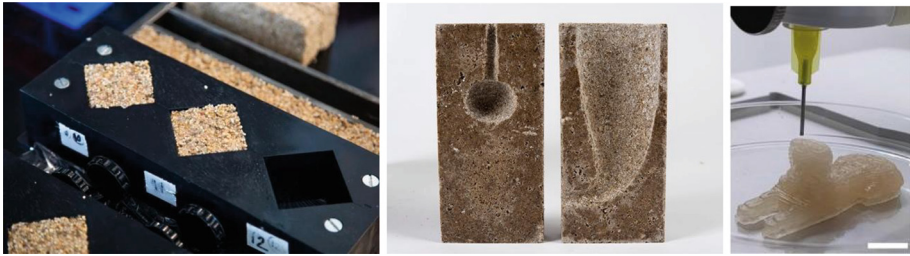
Fig. 4. Left: Sand and a gelatine-based hydrogel mixture in a mould where bacteria are added to create Living Building Material by Heveran, et al. (2020), (retrieved from: colorado.edu), Middle: undercuts and organic shapes inside of a brick in Marmelstein by Paulina Gellert & Anna Herbert (2017) (retrieved from: burg-halle.de), Right: 3D printed bacteria-containing microgel-based ink before the microbial biom mineralisation process of BactoInk by Hirsch, et al. (2023).
