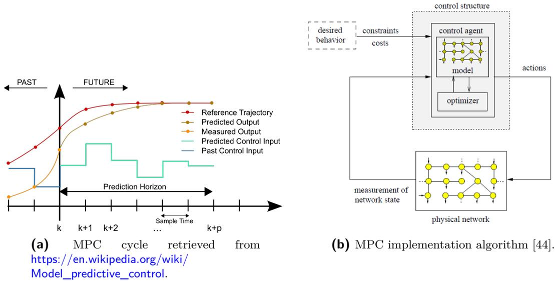
**Figure 3-1:** MPC main principles and implementation algorithm.
