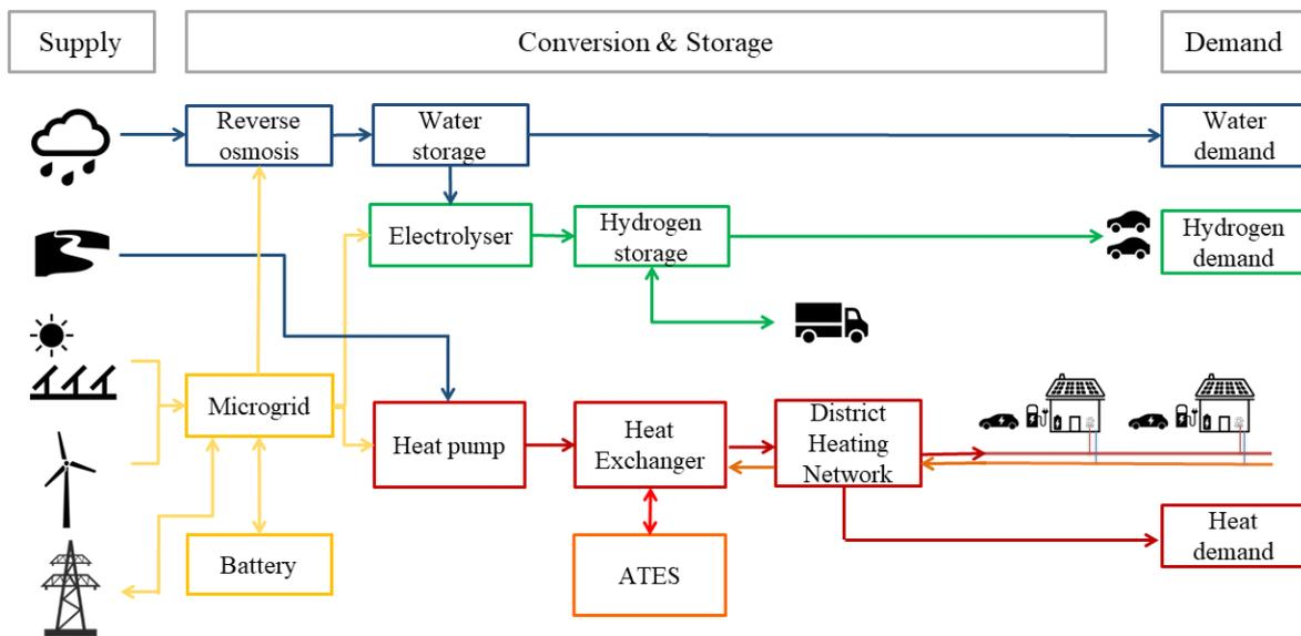
**Figure 2-1:** Schematic energy flow diagram of the Power-to-X system. Energy flows in yellow correspond to electricity, blue to water, and green and red to hydrogen and heat, respectively.
