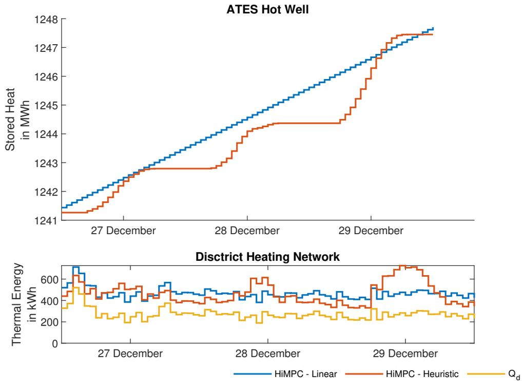
**Figure 3-8:** Comparison of the district heating system in the summer, where the HiMPC - Heuristic controller is driven by PV generation.
