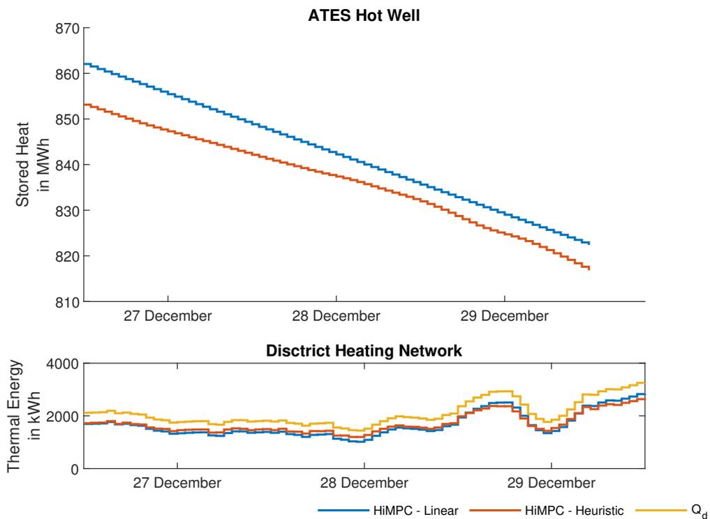
**Figure 3-9:** Comparison of the district heating system in the winter, where the HiMPC - Heuristic MPC is driven by the heating demand.
