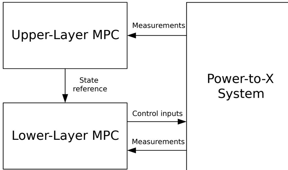
**Figure 3-6:** Proposed HiMPC scheme. Consists of two interacting layers, the UL-MPC providing ATEs hot well reference values for the LL-MPC which acts as EMS
