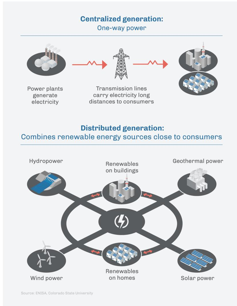
**Figure 1-1:** Centralised and distributed generation in power infrastructures [3].
