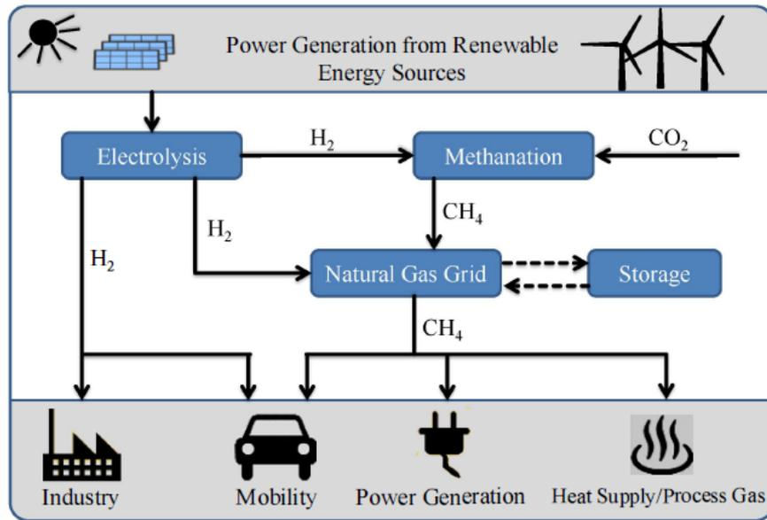
**Figure 1-2:** Typical power-to-gas system based on methane and hydrogen, very obvious is the fact that this system is unwittingly also a power-to-mobility and power-to-heat system [17].
