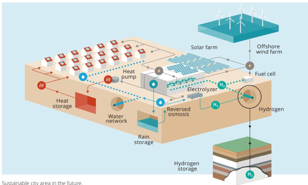
Figure 1-5: Power-to-X system as conceptualised by KWR, including electricity, heat, hydrogen and (demineralised) water supply, demand and generation [30].
