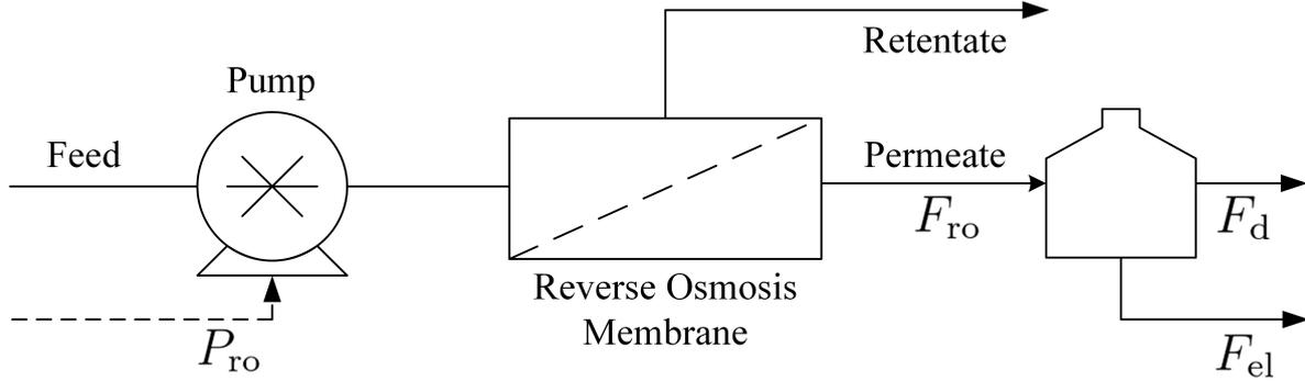
**Figure 2-4:** Reverse osmosis process for purifying rainwater, water flows depicted as solid arrows and electricity as dashed arrows.
