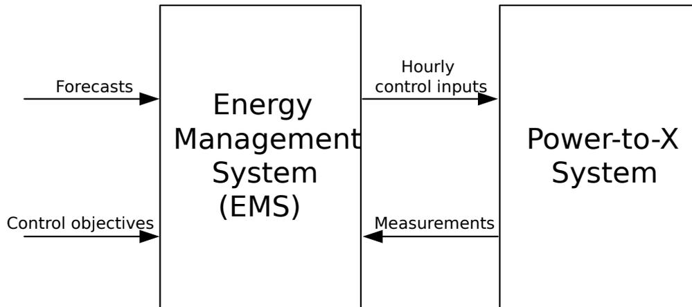
Figure 3-2: Interaction of the EMS with the Power-to-X system.
