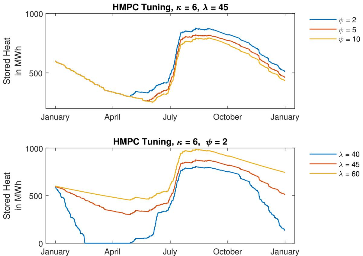
**Figure 3-4:** Tuning of the HMPC control scheme, upper plot varies  $\psi$  and the lower plot varies  $\lambda$  while keeping other parameters constant.
