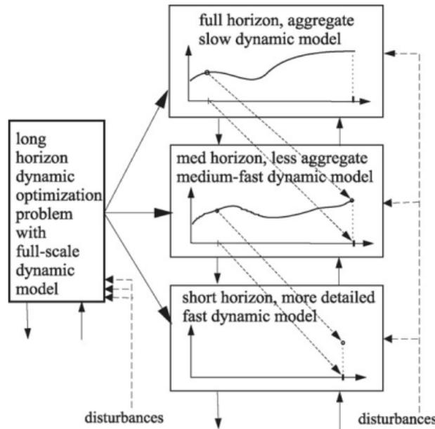
**Figure 3-5:** Example of a time-scale decomposition into three layers [50].
