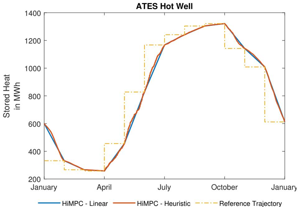
**Figure 3-7:** Comparison of the thermal energy storage of the ATES warm well for a year.
