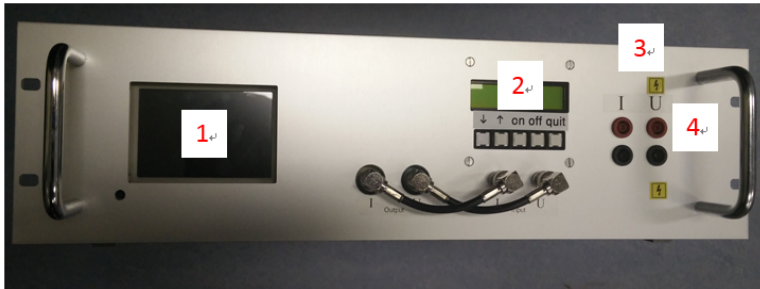
Figure 9.14: Front panel of the dummy load device. 1: waveform display screen. 2: button selecting screen. 3: I port. 4: U port.
