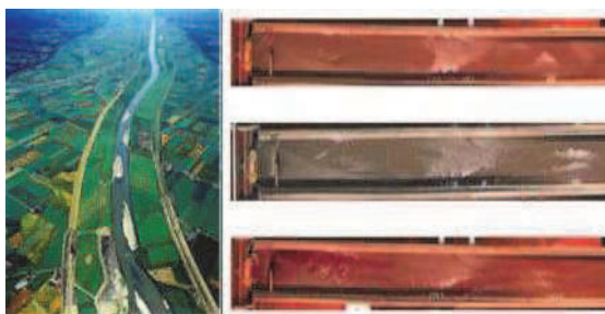
Figure 1 Alternate bars: Rhine River (Left), Experimental flume of Tewolde (2015) (Right)
