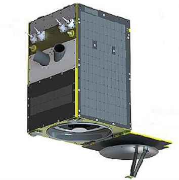
Figure 4.4: The Skysat-3 from Planet's Skysat constellation. In the bottom of the image, an aperture cover that protects the imaging payload during launch is visible. Retrieved from space.skyrocket.de [3]
