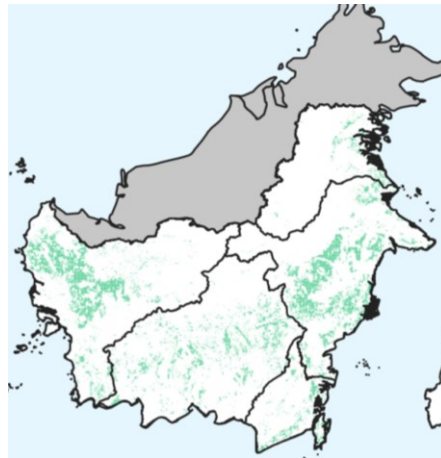
Figure 10 Spatial distribution of suitable areas (green shades) for solar PV in Kalimantan based on geographical constraints according to Pragt (2021).
