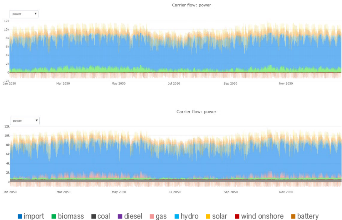
Figure 20 Economic dispatch optimization results for 2050. X-axis = time in 2-hour and Y-axis = MW. Each colour represents different types of power plants. Top: emission-optimized result. Bottom: cost-optimized result.
