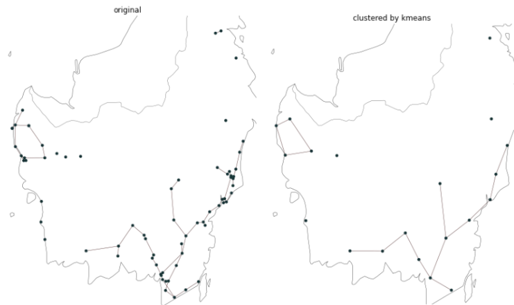
Figure 3 The simplification of the conceptual Kalimantan power system in 2021. Left: the initial conceptual Kalimantan power system. Right: the simplified conceptual Kalimantan power system by k-means clustering.
