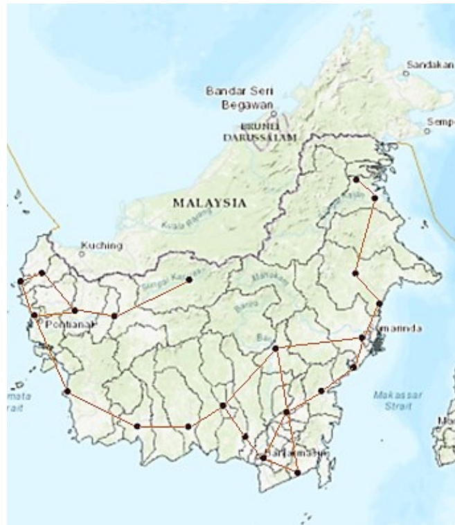
Figure 5 The location of centroids (red dots) and transmission links (orange lines) with respect to kabupaten/kota borders in Kalimantan (black lines) in the 2030 and 2050 conceptual models.
