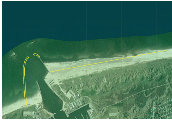
Figure 2.10: Proposed layout of Hvide Sande harbour breakwaters (curved yellow lines) and coastline location obtained with a capital dredge to enhance natural bypass of sediment. (Hillen et al., 2009)
