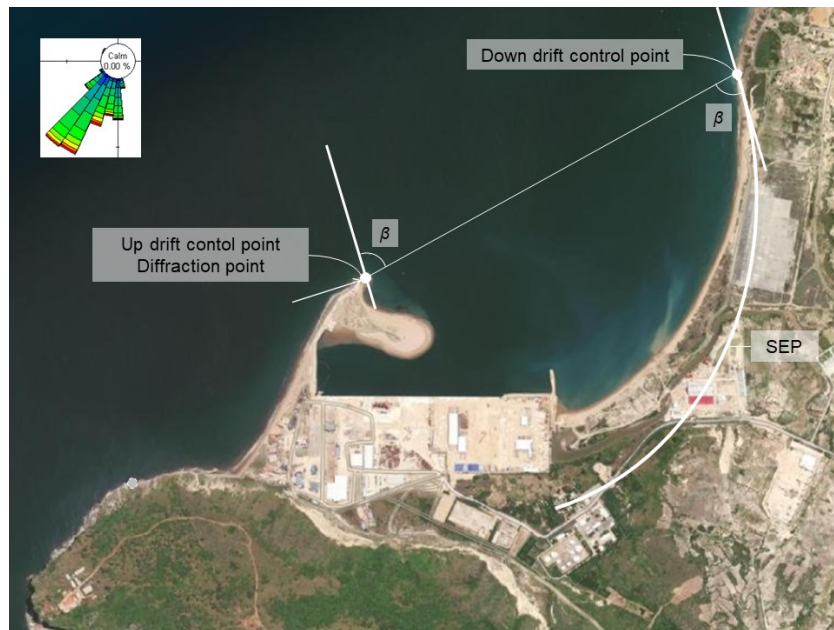
Figure 4.12: Indication of the Static Equilibrium Planform (SEP) of the Bay of Amboim
