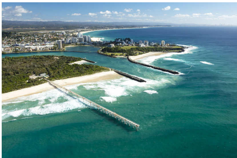
Figure 5.1: Tweed river entrance along the coast and the sediment bypass system (Tweed Sand Bypassing, 2020)
