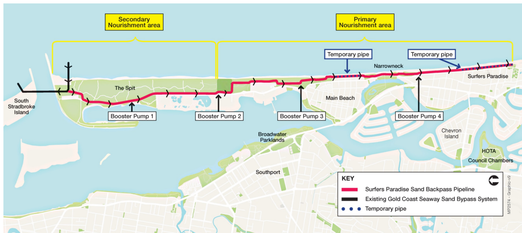
Figure 2.7: Sediment bypass system: Gold Coast Seaway Sand Bypass System and the Surfers Paradise Backpass Pipeline used for sediment management along the Gold Coast beaches and the Gold Coast Seaway. (City of Gold Coast, 2020)
