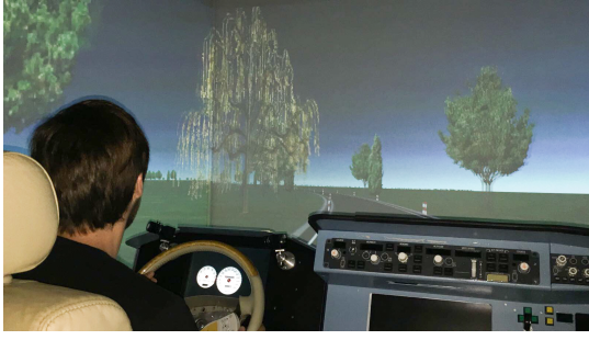
Fig. 4. The fixed-base driving simulator at the Faculty of Aerospace Engineering of the Delft University of Technology.
