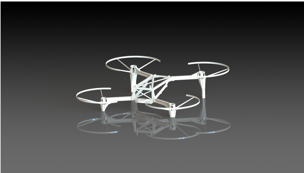
Figure 8.8: Structure of the “DALE” drone before topology optimisation.
