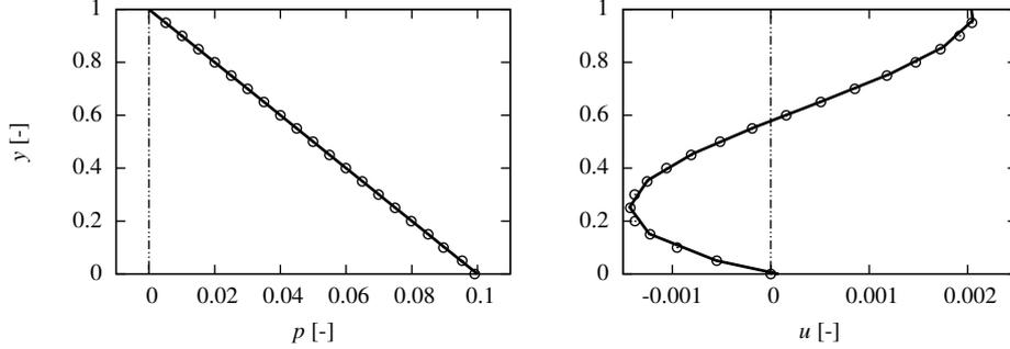
Figure 6: Modified pressure  $p_m$  (left) and horizontal velocity  $u$  (right) for the line  $x = 0$  for  $A = 0.1$ ,  $Re = A$ ,  $Ha^2 = 1$ ,  $Bo = A^2$ ,  $Ca = A^4$  and  $\theta = 90^\circ$ . The numerical simulation ( $\circ$ ) and the first order analytic approximation (solid line) are shown.
