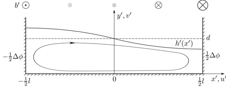
Figure 1: Schematic representation of the liquid layer, with a potential difference  $\Delta\phi$  across the domain and an insulated bottom. The dash-dotted line is the undisturbed interface and the solid line  $h(x)$  is the equilibrium surface position after application of a magnetic field in the direction perpendicular to the  $xy$ -plane, where the relative field strength is indicated in the top.
