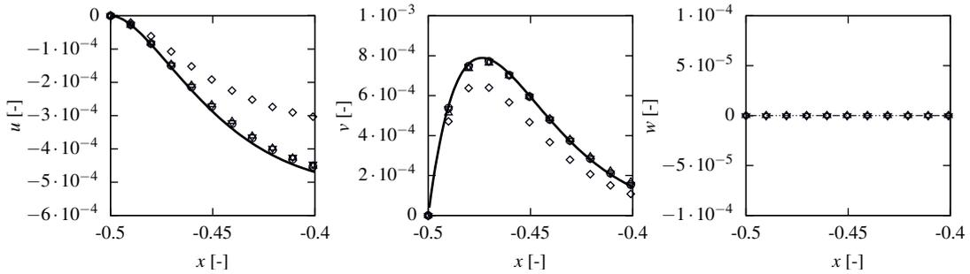
Figure 8: Horizontal (left) and vertical (middle) velocity components (as figure 7) and spanwise velocity component (right), along the line  $y = 0.5$  for  $A = 0.1$ ,  $Re = A$ ,  $Ha^2 = 1$ ,  $Bo = A^2$ ,  $Ca = A^4$  and  $\theta = 90^\circ$ , for the analytical solution (solid line), the two-dimensional numerical simulation ( $\circ$ ), and the numerical simulation for a cavity with  $z$ -dimension  $100d$  ( $\triangle$ ),  $10d$  ( $\nabla$ ) and  $d$  ( $\diamond$ ).
