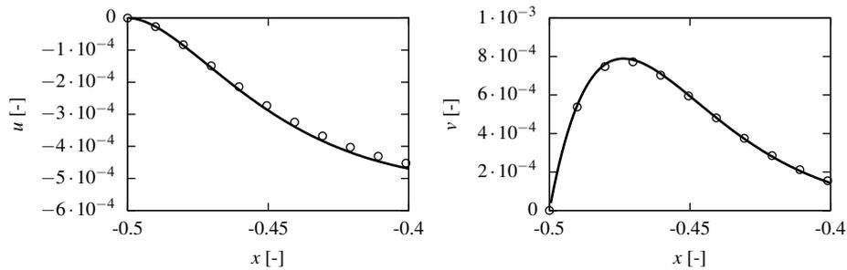
Figure 7: The horizontal (left) and vertical (right) velocity component along the line  $y = 0.5$  for  $A = 0.1$ ,  $Re = A$ ,  $Ha^2 = 1$ ,  $Bo = A^2$ ,  $Ca = A^4$  and  $\theta = 90^\circ$ . The numerical simulation ( $\circ$ ) and the first order analytic approximation of equation 72 using  $P = 1024$  for  $y = 0.5$  (solid line) are shown.
