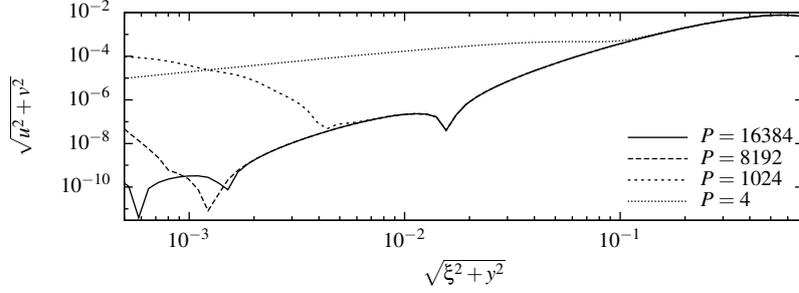
Figure 3: The velocity magnitude along the line  $\xi = y$  in figure 2, which shows the effect of increasing the amount of poles (see equation 72) on the velocity magnitude for  $P = 4$ ,  $P = 1024$ ,  $P = 8192$  and  $P = 16384$ .
