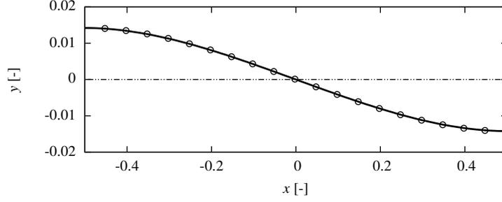
Figure 5: Elevation  $h_2$  of the free surface over the width of the domain for  $A = 0.1$ ,  $Re = A$ ,  $Ha^2 = 1$ ,  $Bo = A^2$ ,  $Ca = A^4$  and  $\theta = 90^\circ$ . The numerical simulation ( $\circ$ ) and the first order analytic approximation (solid line) of equation 61 are shown.
