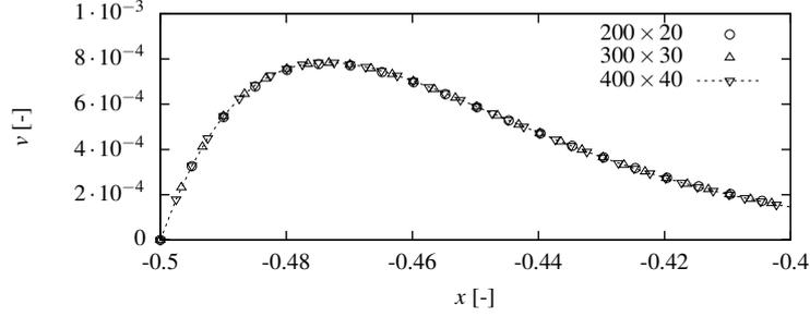
Figure 4: The vertical velocity component along the line  $y = 0.5$  for  $A = 0.1$ ,  $Re = A$ ,  $Ha^2 = 1$ ,  $Bo = A^2$ ,  $Ca = A^4$  for mesh resolutions of  $200 \times 20$ ,  $300 \times 30$  and  $400 \times 40$ .
