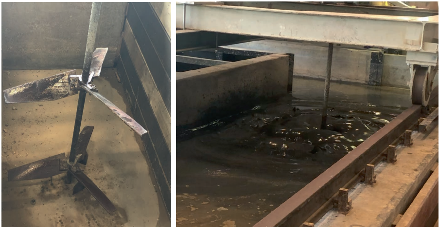
Figure 5.2: The rotating mixer used to homogenise the mud. The right panel shows the mixer in action.
