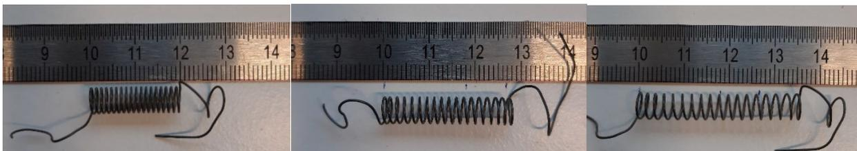
Figure 4.5 The spring forms with 10% deformation (left), 50% deformation (middle), 100% deformation (right).
