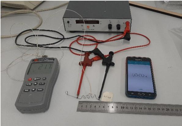
Figure 7.11 Test Setup to measure the response time of the SMA wires
