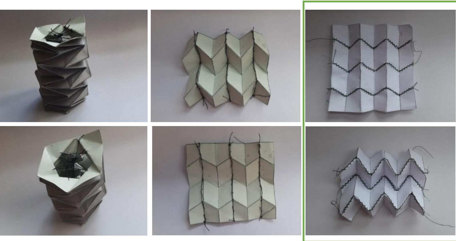
Figure 6.4: Left: Kresling fold with SMA spring in the middle; Middle: Mushi fold with three wires trained to be straight; Right: Mushi fold with three wires to be trained in a zigzag.
