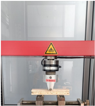
Figure 28: Zwick 3 point bending testing
