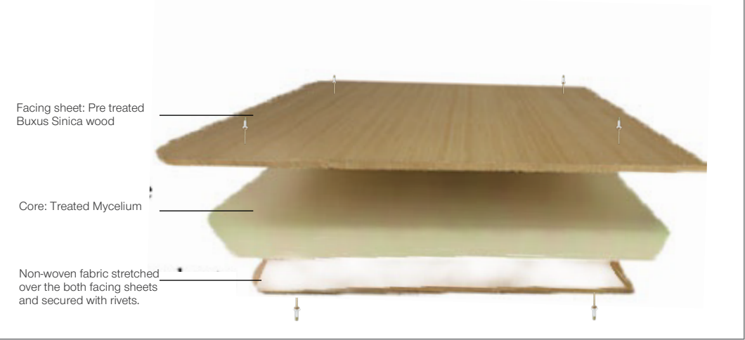
Figure 26: Cross-Sectional View of Composite Structure with Buxus Sinica Wood Facing, Mycelium Core, and Non-Woven Fabric Layer.
