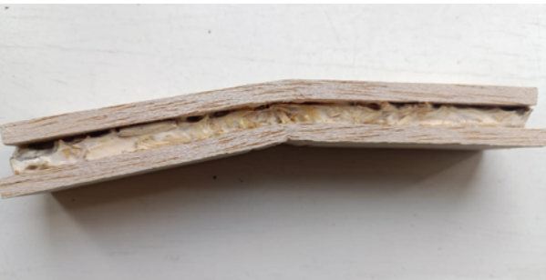
Figure 30: De lamination of the core from the balsa facing sheet
