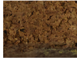
Figure 40: High resolution Images of the MBC+Cork surface following the droplet application
