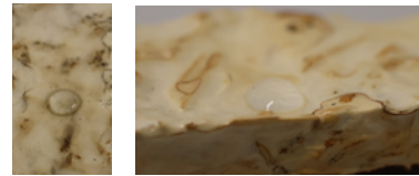
Figure 39: High resolution Images of the MBC+Bio Seal surface following the droplet application
