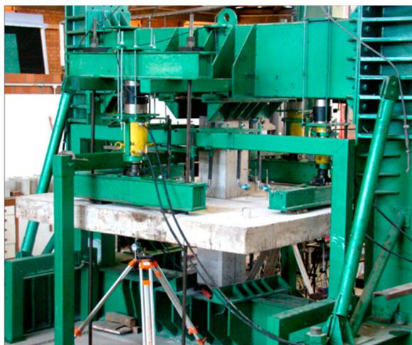
Figure 4. Test setup for series LC by [2].
