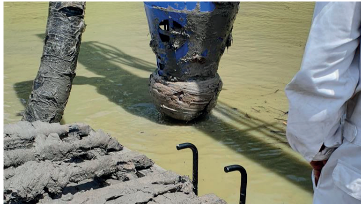
Figure 1. Example of using a cutter head in a highly plastic clay
