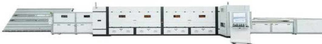
Figure 2-20 Ultra-short pulse laser from Corning Technologies which is capable to manufacture glass substrate of up to 2300mmx2500mm.
