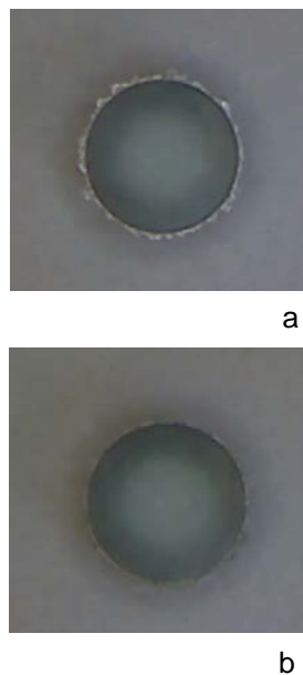
Figure 2-17 Photo taken with microscope of 2mm mechanically drilled hole in 2mm annealed glass pane, a. at the exit of the drill, b. at the entrance of the drill.
