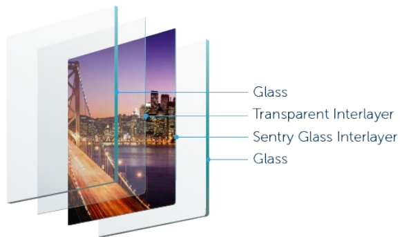
Figure 2-26 Digitally printed image on a PVB interlayer, source: http://coolingbros.com.au/our-products/digiglass/
