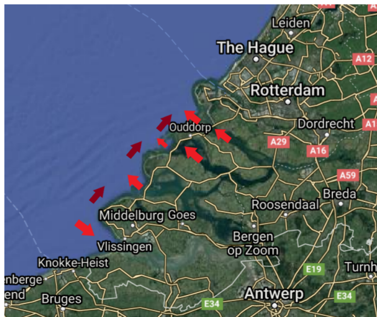
Figure 8: Net yearly directions of the sediment transport (the small arrow indicates a small amount of transport)
