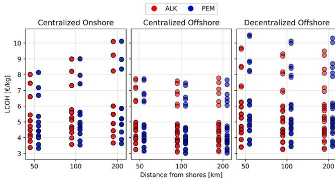
Fig. 5. Range of LCOH found for each system configuration for three wind park sites (characterized by their distance to shore).
