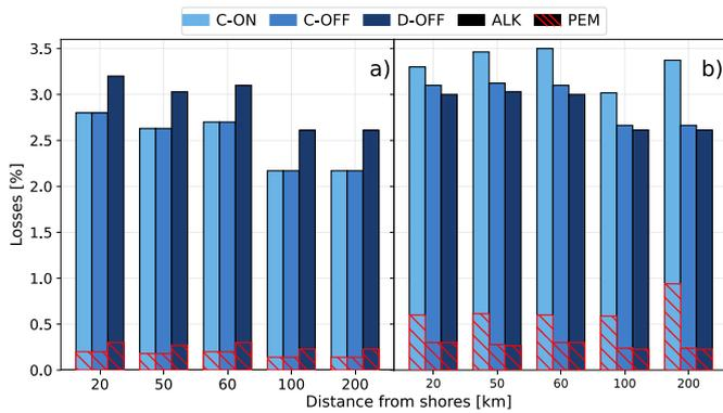
**Fig. 14.** Overview of the operational behavior of the offshore configurations with PEM and ALK with the inclusion of additional wind park sites HKZ (20 km) and IJV (60 km).
