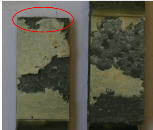
Figure 3.32 Area of Initiation (1mm sample) with visible steel line on top of the outer adherend
