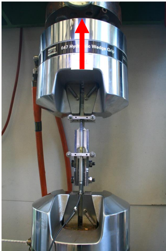
Figure 3.4 25T hydraulic universal testing machine and loading direction
