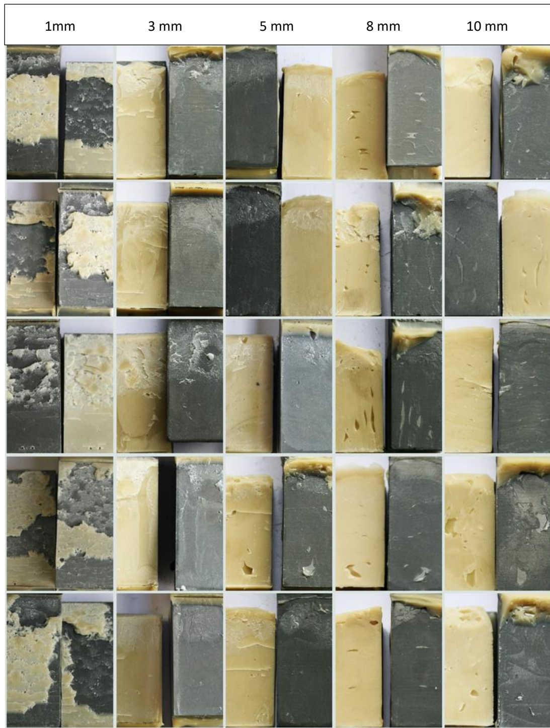
Figure A.2.1. Araldite, failure surfaces of all samples
