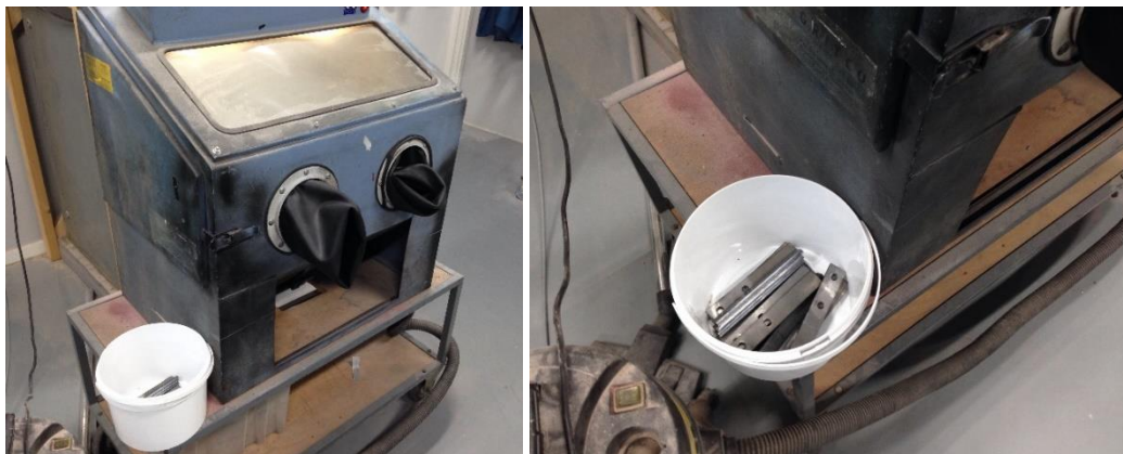
Figure 3.2 Surface preparation of plates. Left: Air pressure machine. Right: Plates after being cleaned with Acetone
