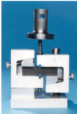
Figure 2.17 V-notched beam test, fixture and specimen according to standard ASTM D 5379 [24]
