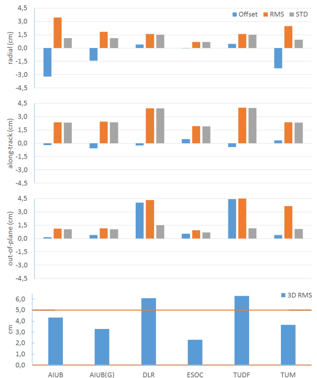
Fig. 3. RSR #2 comparison interval: Mean values (mm) of daily offsets, RMS and standard deviations from comparison between official CPOD orbits and orbits from QWG institutions.
