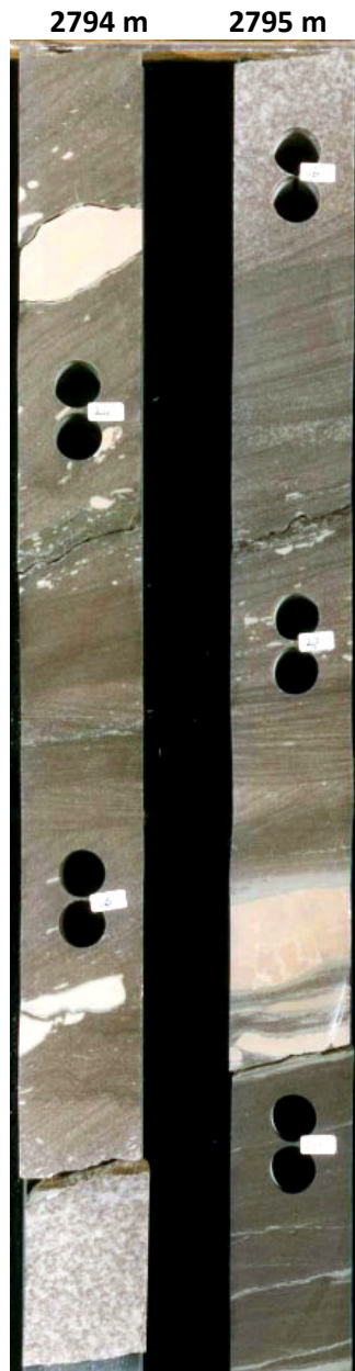
Figure 22: Core photo from well Q13-04 with the expected base of Lower Detfurth. Notice the anhydrite section ~2795m.
