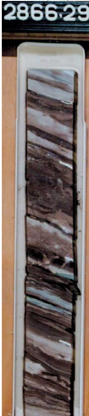
Figure 10: Shale interval of top Lower Volpriehausen with two shale types, well VAL-01
