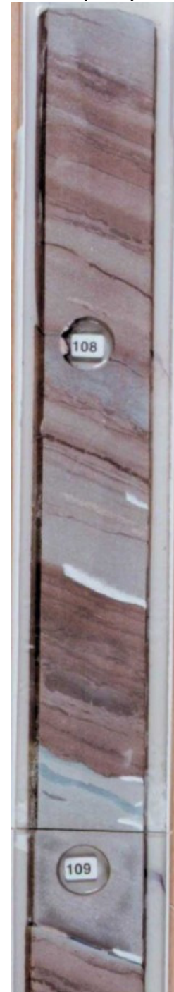
Figure 11: Lower section of Upper Volpriehausen, well VAL-01. Notice the small scale channel erosion surfaces.
