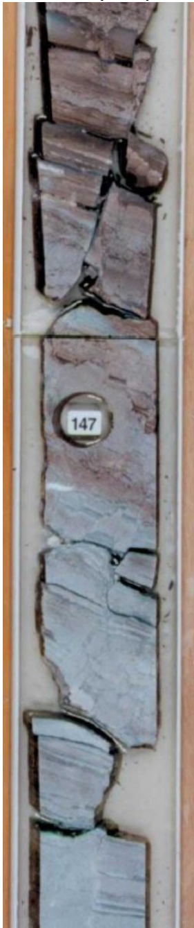
Figure 9: Lower section of shale interval in top of Lower Volpriehausen, well VAL-01. Notice the small scale fractures.
