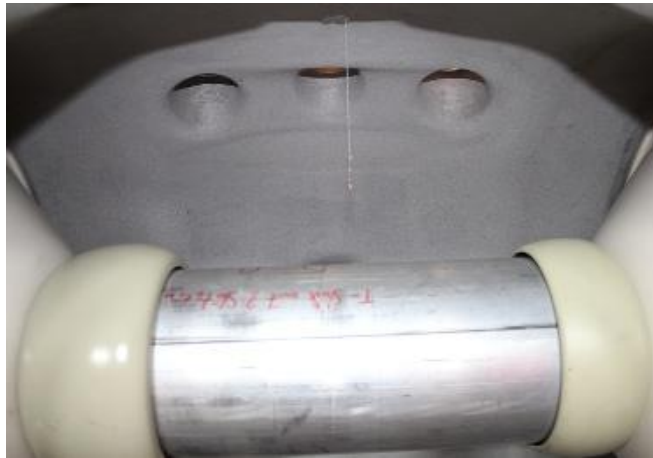
Figure 9.1 The particle placed inside of the test setup in GIS at the High Voltage Laboratory in Stuttgart
