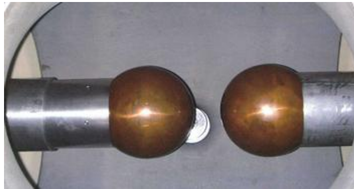
Figure 3.7 The spark gap used in generating the VFTO (on behalf of the Stuttgart University)
