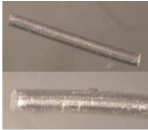
Figure 3.10 An example of aluminum particle used during the investigation under AC Voltage.
