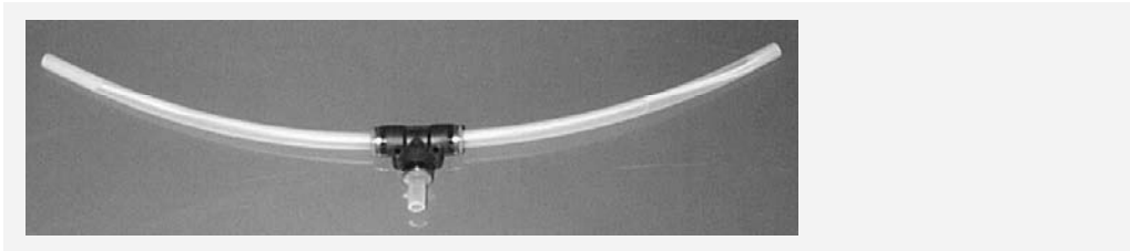
Figure 4.3 Second membrane module with PVC-tube supported membrane for measurement of the filtration curve during dead-end ultrafiltration; this module showed good results and is proposed as the standard module for SUR measurement
