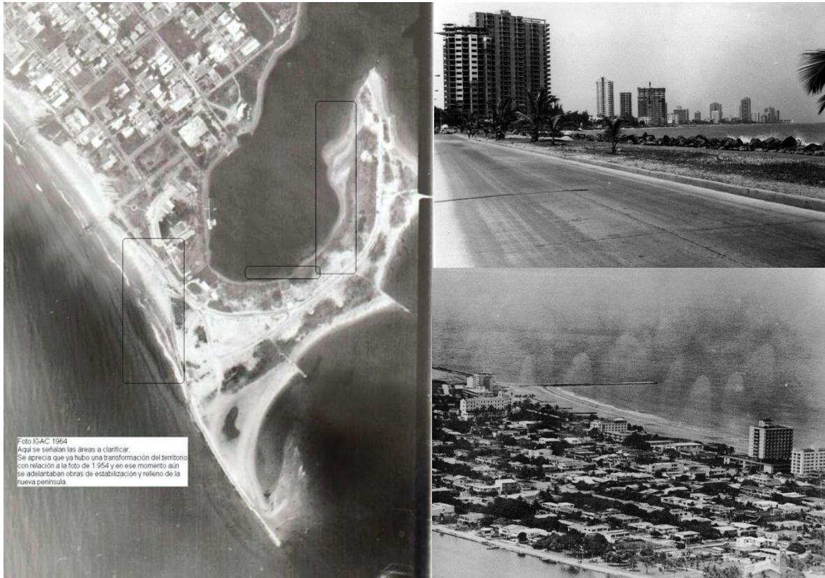
Figure C.18 1964 - Escollera constructed, together with other groynes, more buildings, 1972 start of skyscraper, 1975 completion iribarren groyne
