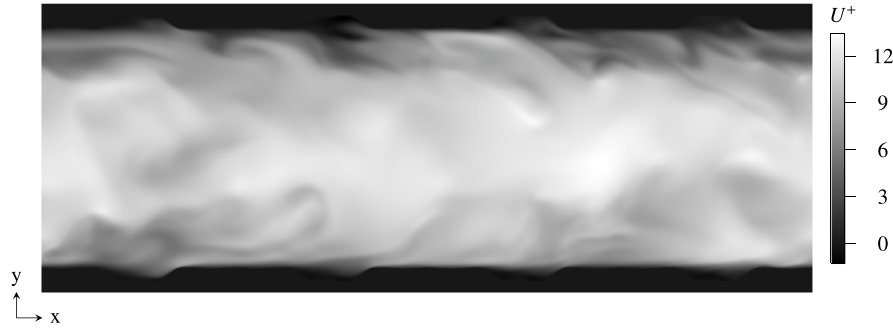
Fig. 13. Instantaneous snapshot of the velocity field in the streamwise direction ( U^+ ) for the highest-performing dimpled surface of the second generation of the reinforcement learning study at Re_\tau = 180 . The slice shown corresponds to the plane at z = L_z/2 . Please note that U = U^+ in our numerical framework. The bulk flow moves from left to right.
