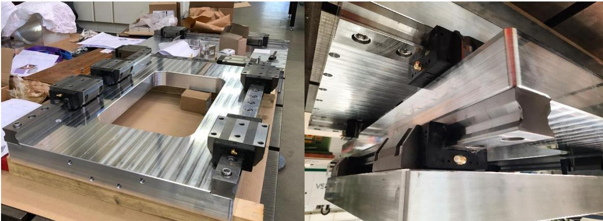
**Figure 4-3:** On the top plate with the first rails attached to it. On the right all three plates with rails in two directions to allow movement in x- and y-direction.
