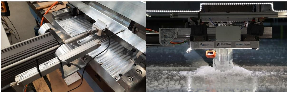
**Figure 4-5:** On the left the side of the setup which stands upside down, with two actuator, load cell and displacement sensor. On the right the total setup combined.
