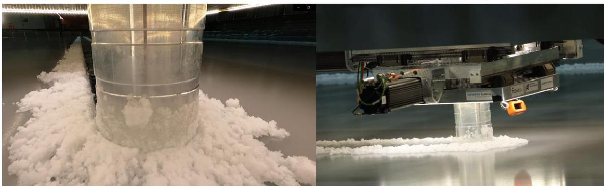
**Figure 4-8:** Two views of the tests at the 15<sup>th</sup> of June with brittle ice characteristics.
