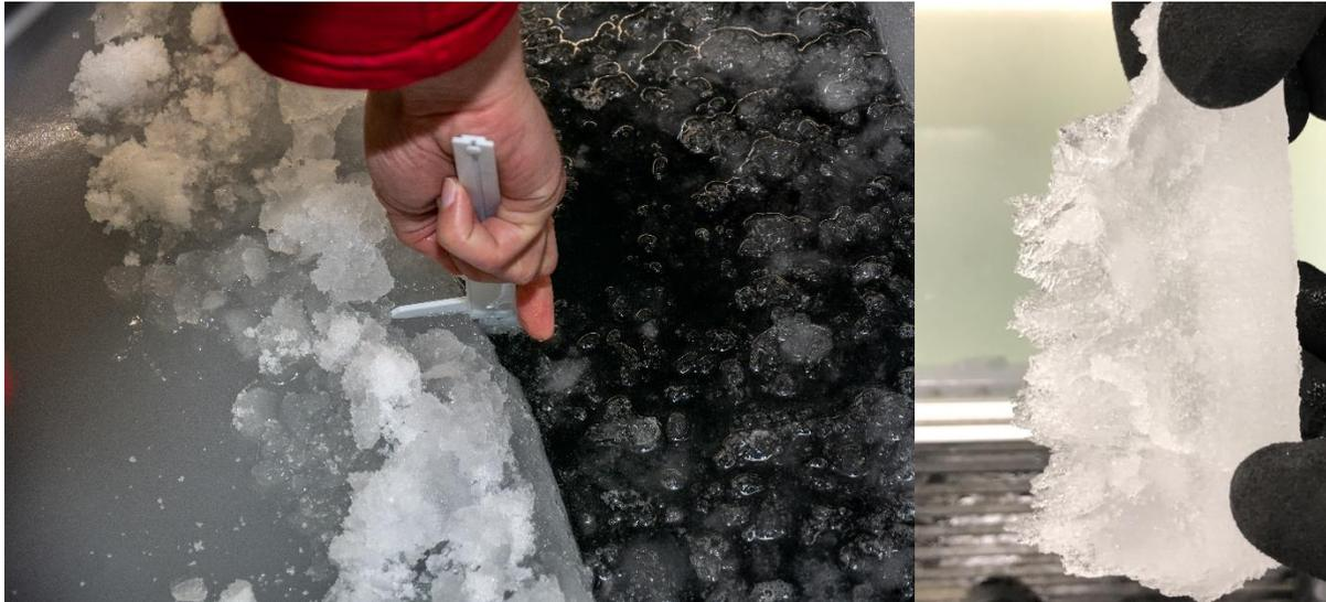
**Figure 6-1:** At the left the measurement method of the ice thickness and on the right a piece from the ice where the variety in ice thickness is clearly visible.
