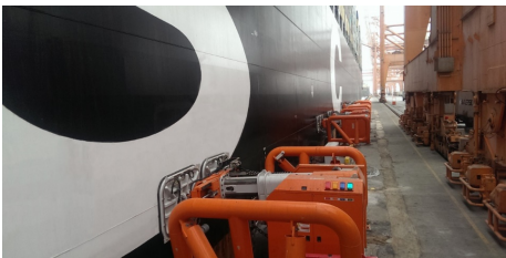
Figure 4.1: Examples of automated mooring systems Left Cavotec's Moormaster [14] and right Macgregor's concept for the Yara Birkeland [47]
