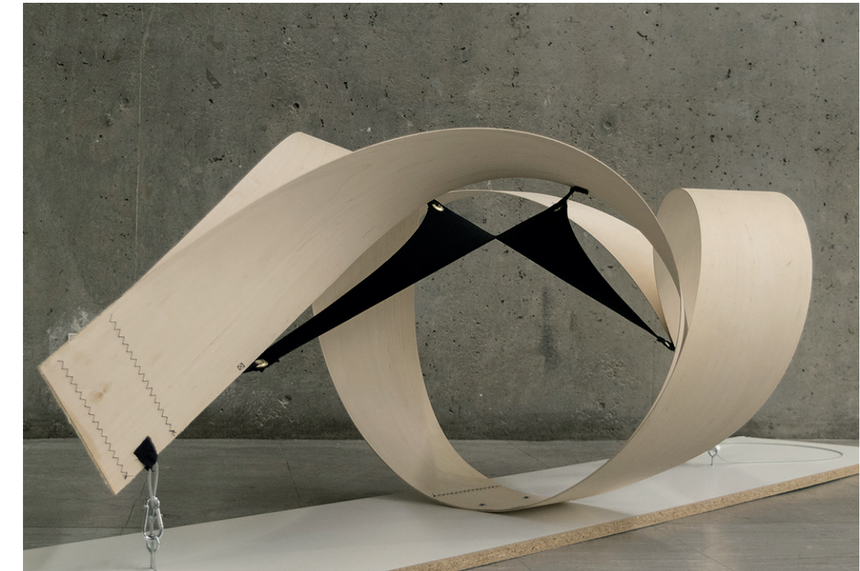
Active-bending structure - torsion research model
