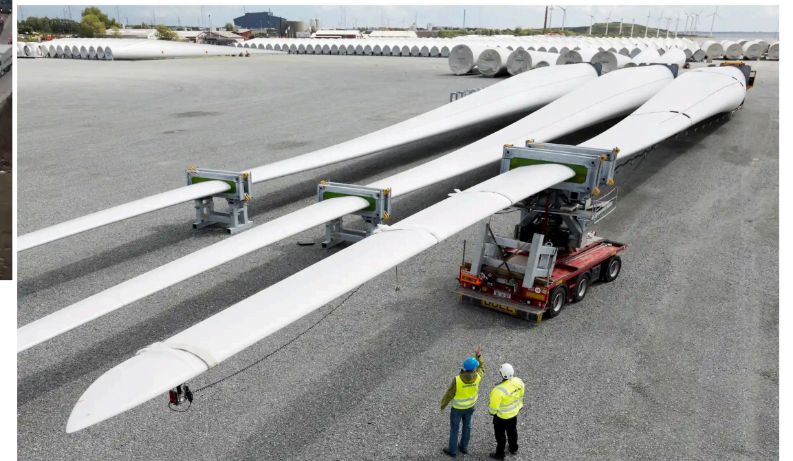
▲ Each wind turbine blade weighs 28 tonnes and is made of balsa wood and fibreglass. Photograph: Paul Langrock/Agentur Zenit/Siemens AG
