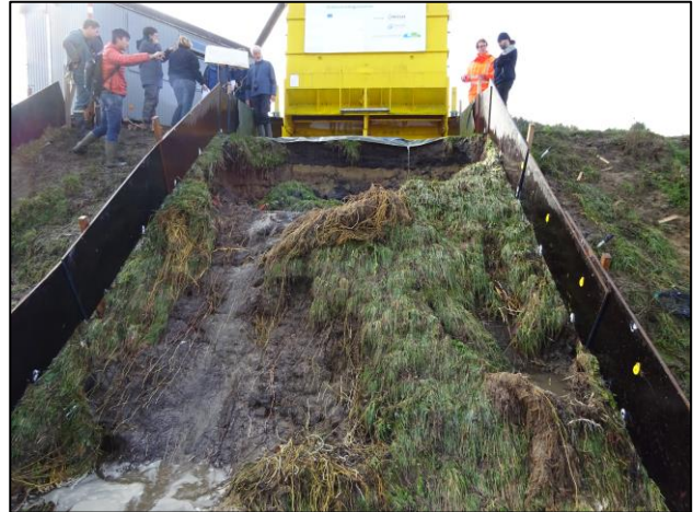
Figure 4. Overview picture taken at the end of the 25 l/m/s tests at the first test section
