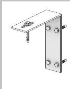
Metal fitting for mounting the prefab element
