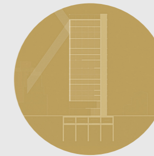
PV + exterior shading in critical locations and openable windows in lower levels for air circulation
