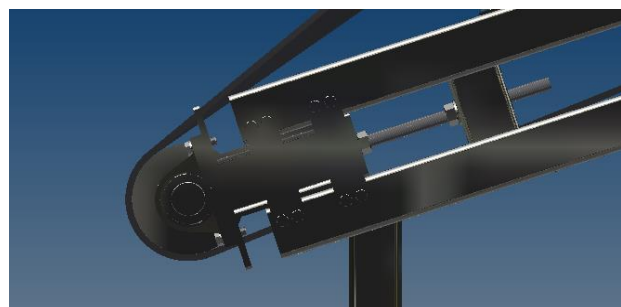
FIGURE 17: BELT TENSIONER AND BEARING
