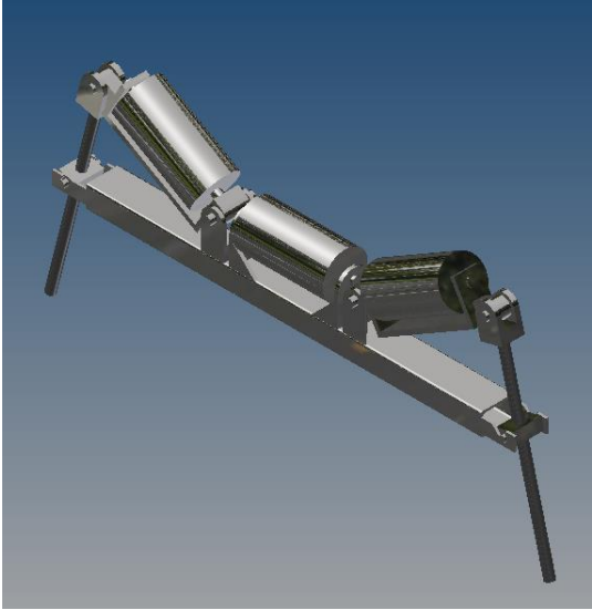
FIGURE 10: ADJUSTABLE IDLER SET AT ANGLE OF 30°
