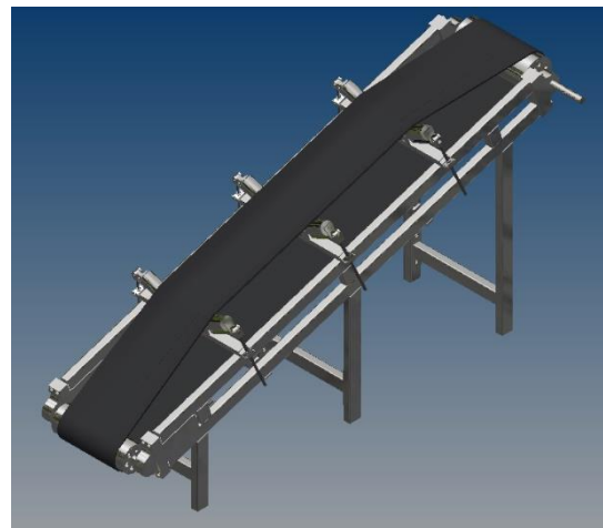
FIGURE 8: DESIGN OF A CONVEYOR WITH A BELT WIDTH OF 400 MM
