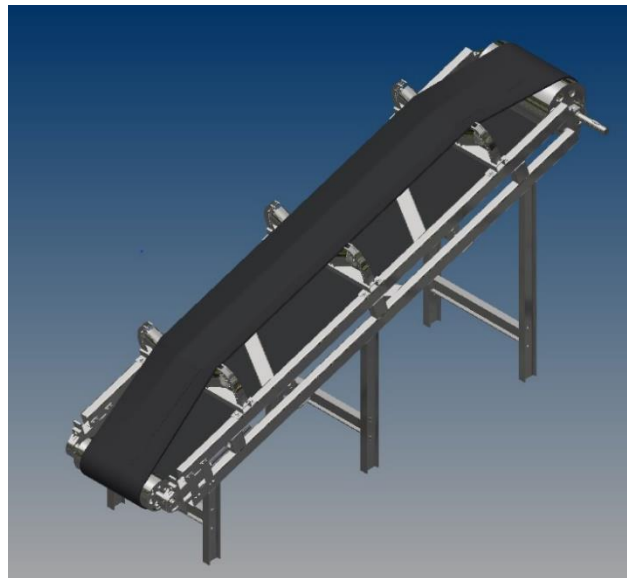
FIGURE 13: THE FINAL DESIGN OF THE CONVEYOR BELT
