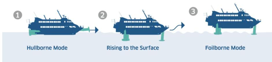
**Figure 1-2:** Operation modes of a hydrofoil craft [24]
