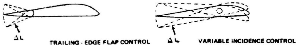
Figure 1-3: Actuators for variable lift force in hydrofoil crafts [35]
