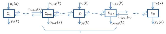
Fig. 1. Illustration of a cluster of subsystems in a neighborhood of the subsystem  $\Sigma_i$  with radius  $R$ . The states  $x_{i-R-1}(k)$  and  $x_{i+R+1}(k)$  are explicitly indicated. They are like all other states unmeasurable.
