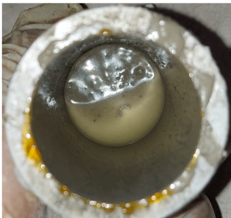
Fig. 11. Drainage of water from the mix for HPMC-free mixtures during extrusion.
